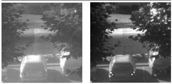
Fig. 11. Example of a dual-band image showing a car in a parking lot with back lights on. (a) longest wavelength image (MWIR2) and (b) short wavelength (MWIR1) image. The device used is grown on CdTe/Ge (2566).
